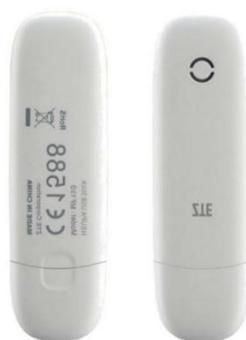
*Fig. 11: Modem 3G ZTE MF626.*
