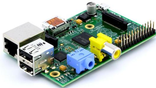
Fig. 10: Raspberry Pi model B.
