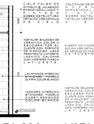
VISTA AMPLIADA 4 S.S #4 APTO.I NIVEL 2, 4, 6 ESCALA: 1:25
