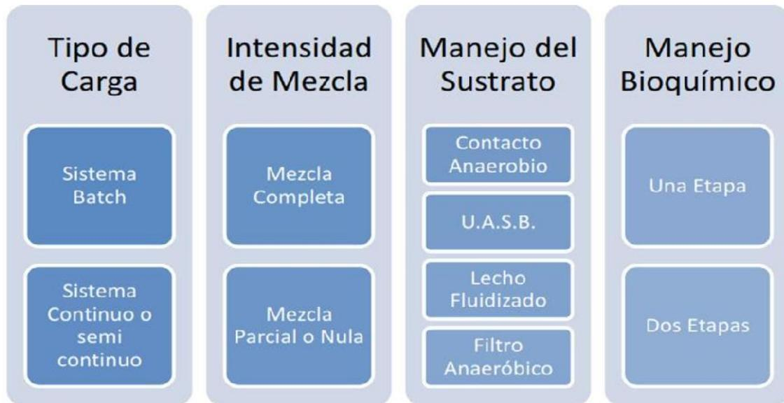
Fuente: Anaerobic digestion process.
