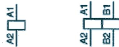
Figura No. 14: Bobinas de control.
