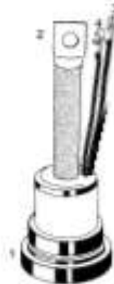
1 = Anode, 2 = Cathode, 3 = Gate, 4 = Auxiliary Cathode
