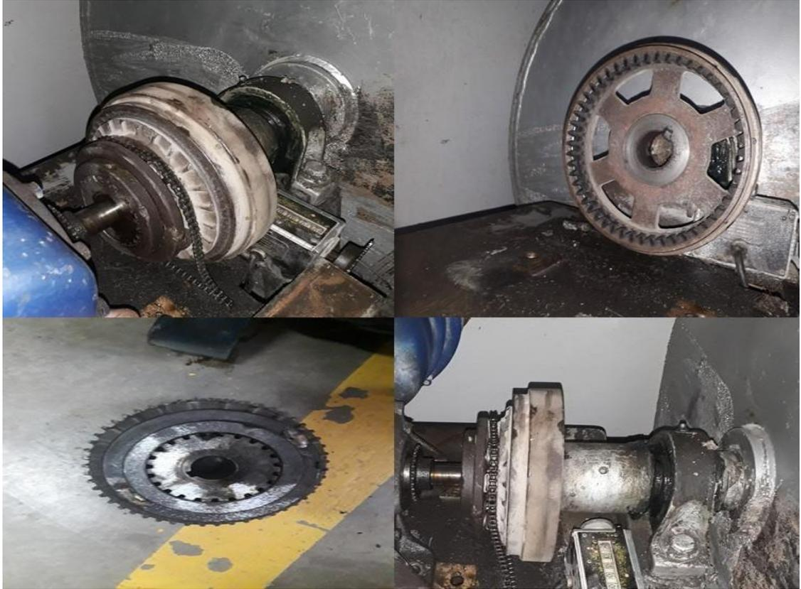
**Figura 18:** Embrague (acople motor – cilindro).
