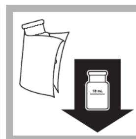
8. Within one minute of adding the reagent, insert the prepared sample into the cell holder with the fill line facing the user. Results are in mg/L Cl<sub>2</sub>.
