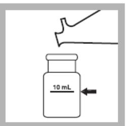
7. **Blank Preparation:** Fill a square sample cell with 10 mL of filtered deionized water from step 6.
