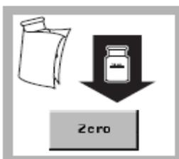
10. When the timer expires, insert the blank into the cell holder with the fill line facing the user. Press **ZERO**. The display will show:
