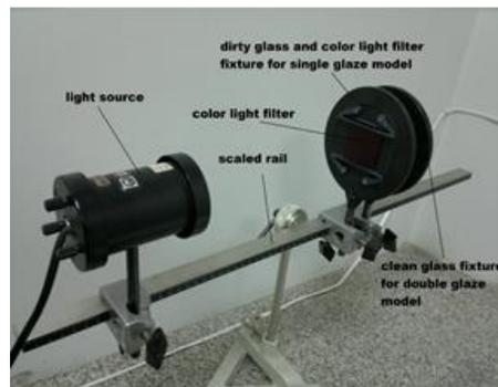
Figure 4 : The scaled rail with glass fixtures.
