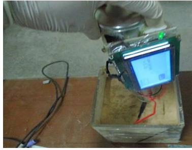
Figure 9. Impact test in the horizontal direction
