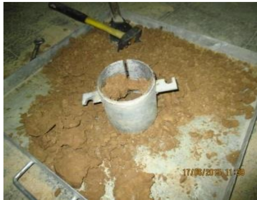
Figure 4. Soil compaction test
