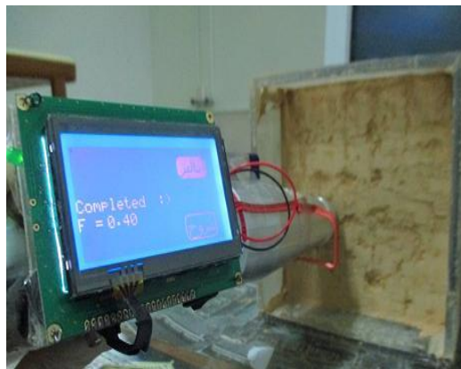
Figure 2. The testing of Electronic rebound hammer device 2-1-1. The device's operation
