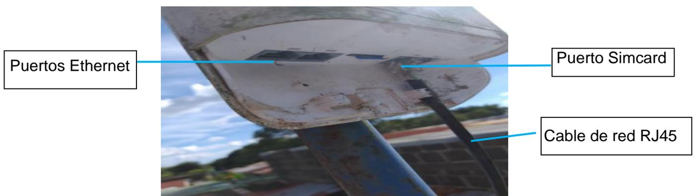
Fig. No. 28 Parte Exterior del CPE Outdoor LTE-TDD cat 6
