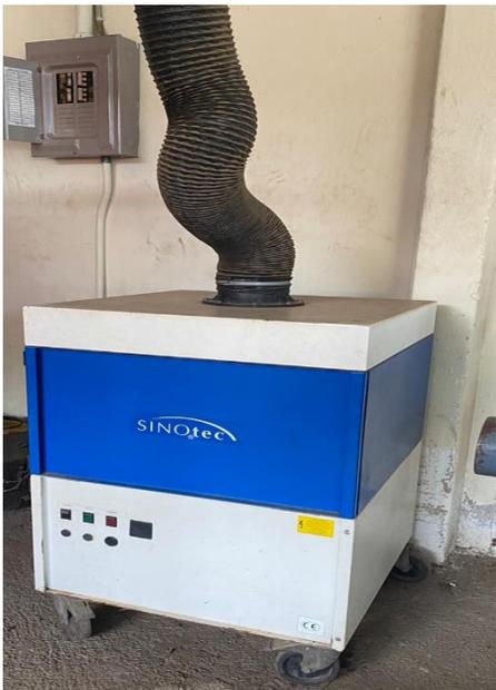
A photograph of a Sinotec gas extractor machine. The machine is rectangular, with a white top and bottom section and a blue middle section. The brand name 'SINOTEC' is visible on the blue section. It has a control panel on the front with several buttons and a power switch. A flexible black duct is attached to the top of the machine. The machine is on wheels and is positioned in a room with a light-colored wall and a grey electrical box on the wall behind it. |
