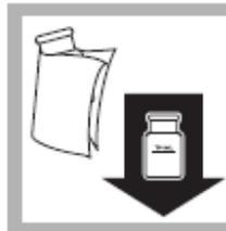
8. Within one minute of adding the reagent, insert the prepared sample into the cell holder with the fill line facing the user.
