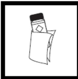
23. Wipe the reagent blank with a damp towel, followed by a dry one, to remove fingerprints or other marks.
