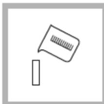
7. Blank Preparation: Rinse a clean 1-cm quartz cell several times with Organic-Free Reagent Water. Fill the cell with Organic-Free Reagent Water. Wipe the cell walls thoroughly.
