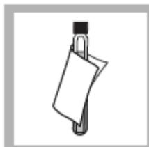
16. Wipe the sample vial assembly with a damp towel, followed by a dry one, to remove fingerprints or other marks.
