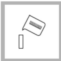
10. Discard the contents of the blank cell and rinse the cell several times with filtered sample. After rinsing, fill the cell with filtered sample. Wipe the cell walls to remove fingerprints.
