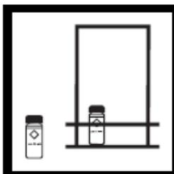
11. Place sample cell in the cell holder assembly. Set the blank aside.
