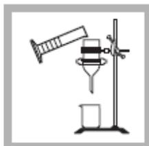
5. Prewash the filter assembly by pouring at least 50 mL of Organic-Free Reagent Water through the filter. Discard the filtered water. Pre-rinsing removes any soluble impurities from the filter.
