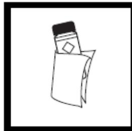
26. Wipe the sample cell with a damp towel, followed by a dry one, to remove fingerprints or other marks.
