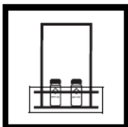
17. Replace the cooling water with fresh, cold tap water. Place the assembly containing the sample and blank cells into the cooling bath.
