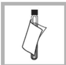
13. Wipe the reagent blank with a damp towel, followed by a dry one, to remove fingerprints or other marks.
