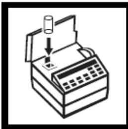
27. Place the prepared sample into the cell holder. Close the light shield.
