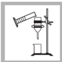
6. Prepared Sample: Pour 50 mL of sample through the filter and collect the filtered sample.
