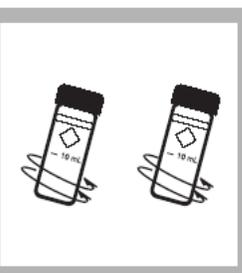
8. Cap tightly and mix gently by swirling each cell three times.
