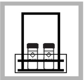
**17.** Replace the cooling water with fresh, cold tap water. Place the assembly that contains the sample and blank cells into the cooling bath.
