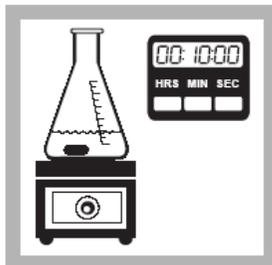
4. Place the flask on a stir plate and stir at a moderate speed for 10 minutes.
