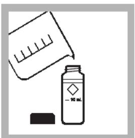
6. **Blank Preparation:** Fill the second sample cell with deionized water. Cap and label as “blank”.
