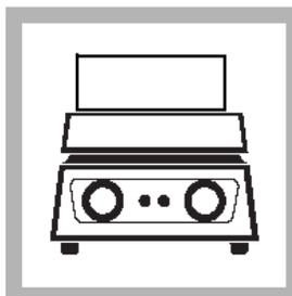
3. Prepare a hot water bath by adding 500 mL of water to an evaporating dish. Put the dish on a hot plate and turn the heater on high.
