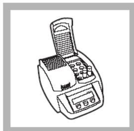
10. Cap the vial assemblies tightly and insert them in the COD reactor for 2 hours at 103–105 °C.
