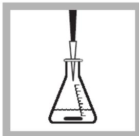
3. Add 0.4 mL of Buffer Solution, pH 2.0. Use pH paper to make sure the sample pH is 2.
