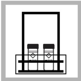
**14.** When the timer expires, remove the assembly and sample cells from the hot water bath. Place in the cooling bath.
