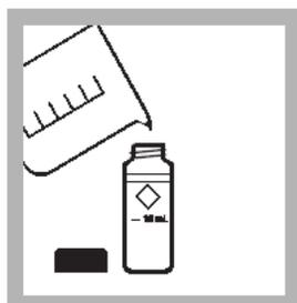
5. **Prepared Sample:** Fill one round sample cell to the 10-mL mark with sample. Cap and label as “sample”.
