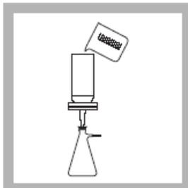
5. Rinse the filter by pouring about 50 mL of deionized water through the filter. Discard the rinse water.
