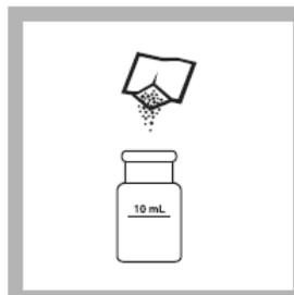
4. **Prepared Sample:** Add the contents of one DPD Total Chlorine Powder Pillow to the sample cell.
