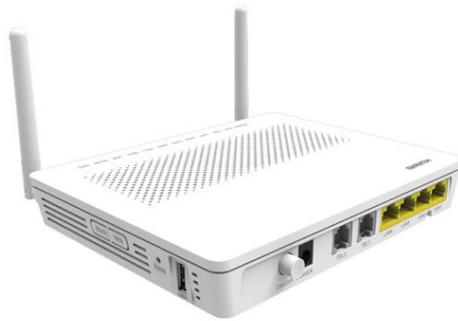
Figura 39: ONU Huawei HG8245H GPON
