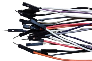
Fig. 23: Cables jumpers. (Fuente Propia)
