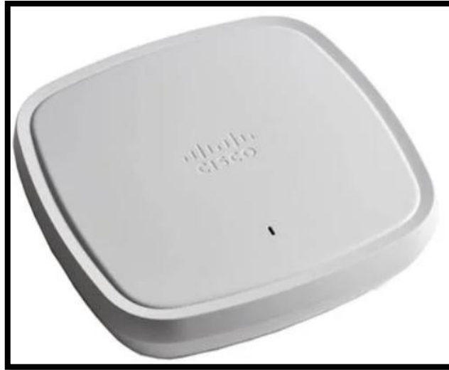
Figura No. 38 Access Point Catalyst 9120AXP-B. [21]
